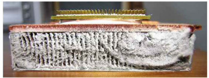
▲ The CPU and cooler from a laptop after three years of operation. With this level of dust ingress, this machine would be very unlikely to reach four years' use, without intervention
